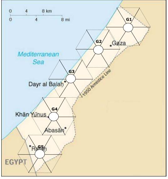
Figure 9 shows the WiMAX network design for Gaza Strip.
