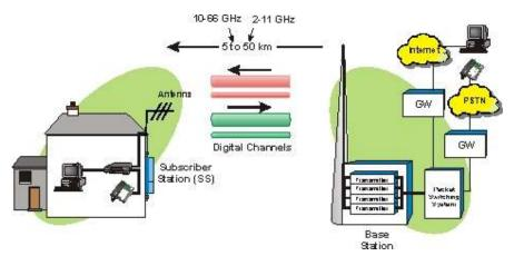
Figure 8: A typical WiMAX Scenario to be used in the GUS (Gaza/West Bank) project.
