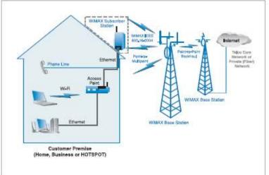
Figure 1: WiMAX Network Topology for Fixed Access Usage Model
